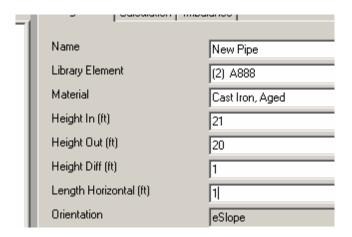
Figure 10: Vertical Pipe Entry Fields
