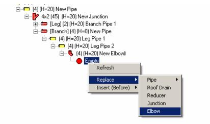
Figure 12: Entering an Elbow
