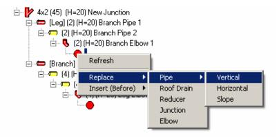
Figure 9: Entering a Pipe Element
