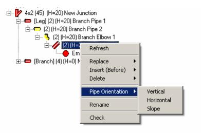
Figure 11: Changing Pipe Orientation
