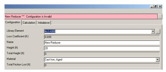
Figure 14: Reducer Configuration Fields
