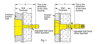
**NOTE:** When ordering, specify Figure Number and "A" dimension. "A" should always be greater than wall thickness for non-freeze installations. When a wall clamp is specified, add 1 1/4" to the wall thickness to arrive at a minimum required "A." The "A" specified should be the next larger, even number; such as 6", 8", 10", etc. Wall hydrants are furnished in lengths of 2" increments.
