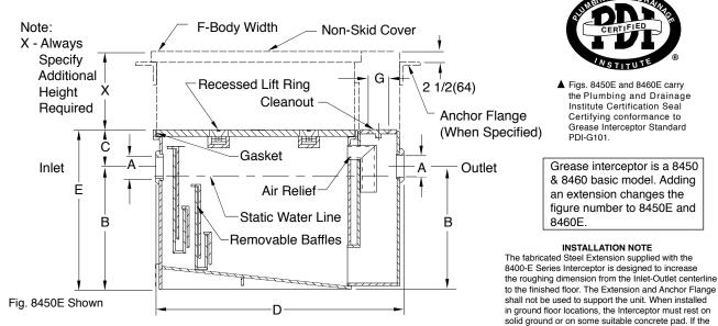
WHEN ORDERING, SPECIFY HEIGHT REQUIRED FROM TOP OF INTERCEPTOR TO TOP OF EXTENSION USING SUFFIX NUMBER FOR EXTENSION HEIGHT. EXAMPLE: FIG. 8460E WITH 6"(150) EXTENSION - SPECIFY FIG. 8460 (-E06)
