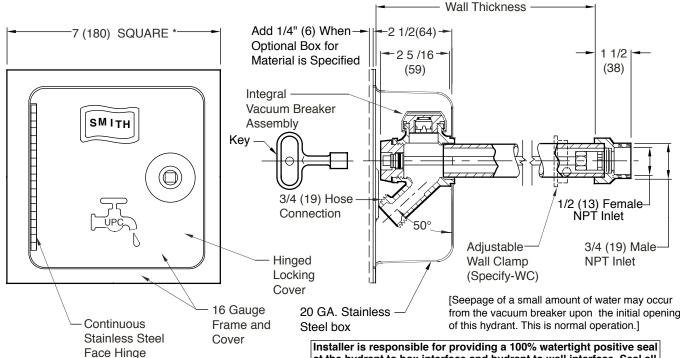
at the hydrant to box interface and hydrant to wall interface. Seal all interior joints, seams, gasket seams/closures including around the hydrant box flange with an appropriate sealant recommended by a sealant manufacturer. NOTE: Jay R. Smith does not warrant the performance or life expectancy of the sealant material.
