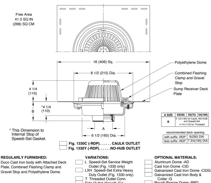
Duco Cast Iron body with Attached Deck Plate, Combined Flashing Clamp and Gravel Stop and Polyethylene Dome.
