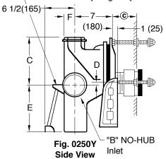
Finished Wall (180)(180)1 (25) Neoprene Face Plate Gasket 4" (100) Adjus-to-Wall Coupling Closet Outlet Gasket Thrust Bearing **Nuts and Washers** Base Support
