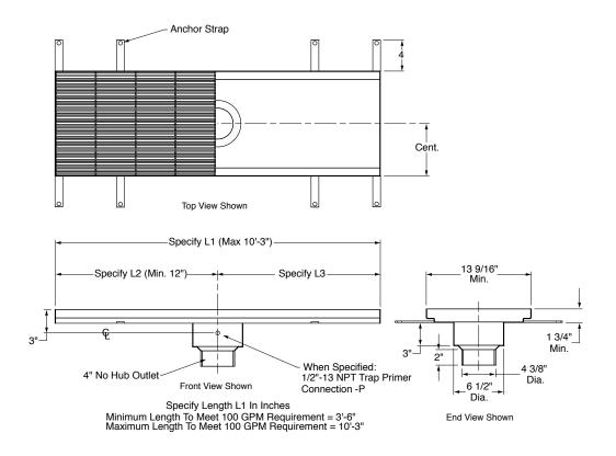
**Option A** - without flange **Option B** - flange w/clamping collar and weep holes
