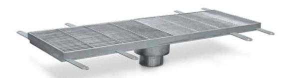
The Jay R. Smith Mfg. Co. Figure number 9679 Threshold Drain<sup>™</sup> is engineered to be in compliance with current building codes addressing fire service access elevators that require protection from water that could enter the elevator shaft during a fire. The 9679 threshold drain is certified to flow 100 gpm with an ADA compliant grate. The threshold drain can be manufactured to custom lengths to meet facility requirements.
