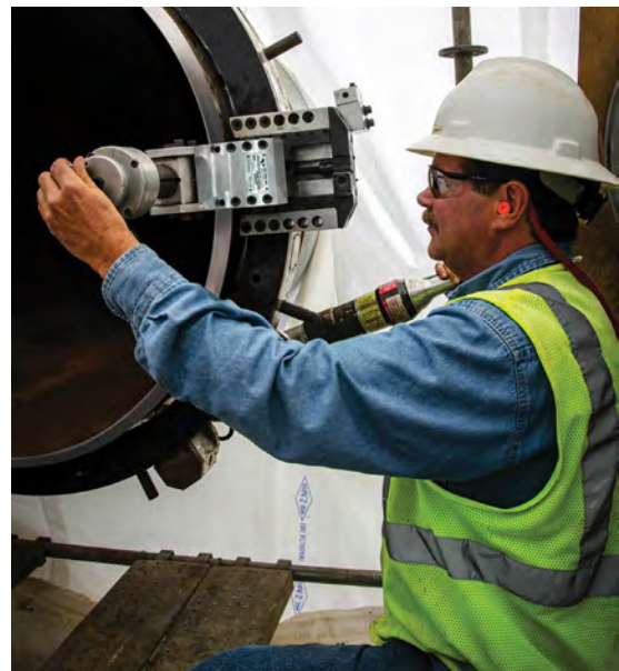
Top: Sauer Group cut costs and stayed on schedule thanks to Tri Tool, which redesigned a torch head to perform the large-bore eccentric I.D. weld overlay, counterbore, weld prep, and finished weld in under 36 hours from identification to weld-out.
