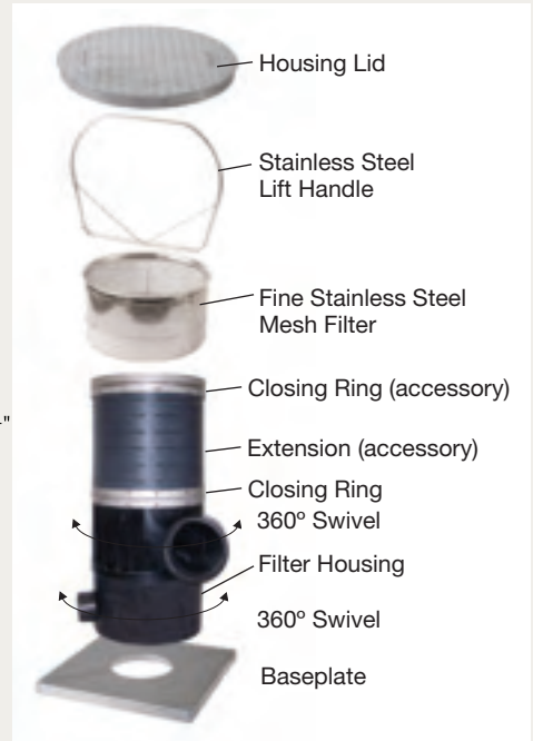
Figure Number: RH9521-12 – 12" Sewer and Drain Outlet, Steel Lid Carries Traffic Loads Up to 12 Tons (DIN 1072/SLW12) Figure Number: RH9521-12XH – 12" Sewer and Drain Outlet, Steel Lid Carries Traffic Loads Up to 60 Tons (DIN 1072/SLW60) Figure Number: RH9521-12AC – 12" Sewer and Drain Outlet, Aluminum Lid for Light Traffic Areas (DIN 1989/SLW3)
