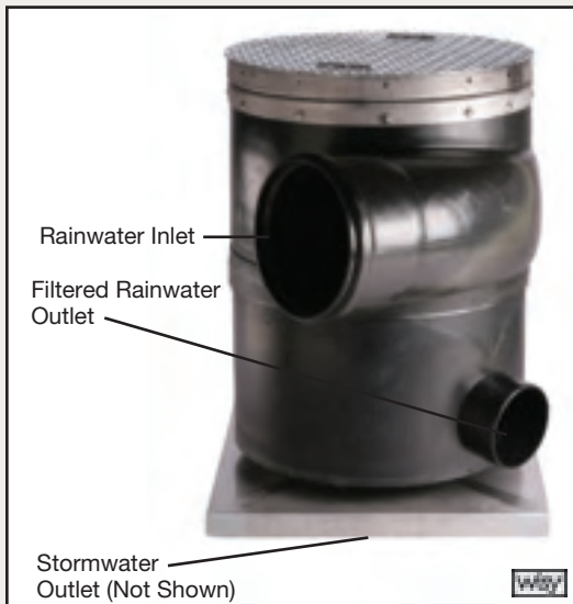
Figure Number: RH9521-12 – 12" Sewer and Drain Outlet, Steel Lid Carries Traffic Loads Up to 12 Tons (DIN 1072/SLW12) Figure Number: RH9521-12XH – 12" Sewer and Drain Outlet, Steel Lid Carries Traffic Loads Up to 60 Tons (DIN 1072/SLW60) Figure Number: RH9521-12AC – 12" Sewer and Drain Outlet, Aluminum Lid for Light Traffic Areas (DIN 1989/SLW3)
